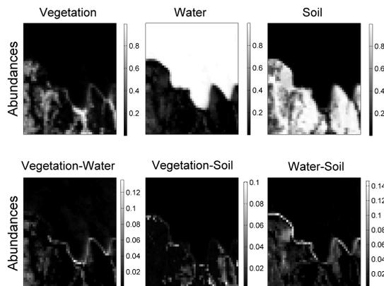
**Fig. 2.** Fraction maps estimated using GBM for Moffett Field.**Table 3.** Unmixing performance for a real AVIRIS image.
